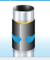
For mechanical protection apply MarineProtect®-100 Jacket. If the coating area of the pile is higher than 1.9 m several jackets may be used. Start mounting the lower jacket. We recommend to install the shorter jacket first. Prepare the Smart<sup>®</sup> Band sections (circumference + min. 5 cm) per Jacket. The length of the jacket allows a sufficient overlap. The overlap of the jacket should not face the breaking waves.
