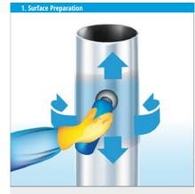
Prepare the surface carefully. Remove all rust, loose particles and loose residues of old coatings from the surface of the pile. Remove any organic substances from the surface. fter cleaning the surface, proceed immediately with the coating to avoid the development of rust and organic growth. We recommend, whenever possible, to use sand or water blasting to gain best results.
