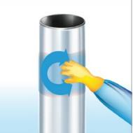
Apply MarineProtect®-Primer on the cleaned surface by hand, roller or using a spreading tool. Make sure that the complete surface is coated with MarineProtect®-Primer. The consumption of MarineProtect®-Primer is about 350 g/m².
