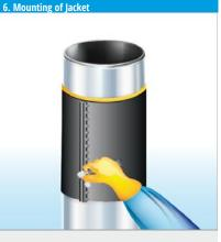
When the MarineProtect®-2000FD Jacket is fastened with all screws, an additional jacket can be mounted above the first one. Position the upper jacket with an min. overlapp of approx. 30 mm. The bars of both jackets can be placed right above each other. The mounting of the upper jacket is then carried out as described in point 5.
