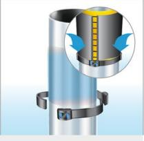
**Optional:** In case of coating a section of the pillar with a distance to the sea ground, a Smart® Band may be used below the first Jacket as a mechanical support. Use three Smart® Band stripes and three standard Smart® Band Buckles to form a ring as indicated in the picture. Fasten the Smart® Band with the SM-FT 2000 or SM-FT 1000 mounting tool.
