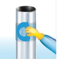
Apply MarineProtect®-Primer on the cleaned surface by hand, roller or using a spreading tool. Make sure that the complete surface is coated with MarineProtect®-Primer. The consumption of MarineProtect®-Primer is about 350 g/m<sup>2</sup>.
