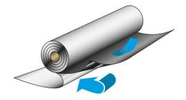
4. Applying slight tension, push the roll in the laying direction while pulling off the separating film. After laying, push the strip down onto the surface using a brush or a small roller.
