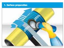
Remove loose coating, smooth out grooves and hollows.
