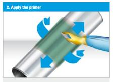
Apply a thin layer of **DENSO® Primer** using your hand or a palette knife onto the steel surface and the adjacent coating. If applying to a wet surface, firmly press the **DENSO® Primer** to remove the moisture from the surface. Material consumption: Average 500 g/m²
