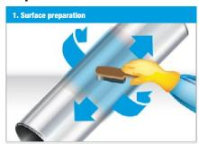
The surface must be free of dust, ice, frost and any loose particles. Rust must be removed with a metallic brush.
