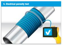
After the application of the **DENSOLEN®** tape it is possible to carry out a test using an electrical porosity controller, provided for in standard. It is recommended to use spiral electrodes or rubber.
