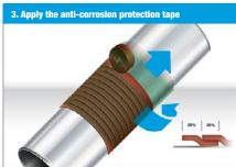
Apply the **DENSO®-Tape** to the pipe in a spiral with 50% of covering and without folds. Smooth the **DENSO®-Tape** by hand and apply firm pressure.
