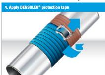
Apply the DENSOLEN®-AS50 (VivaxCoat®-LT/-MT) or DENSOLEN®-ET100 (VivaxCoat®-HT) mechanical protection tape on top of the anti-corrosion tape, with a cover rate of 50% (1x50% of covering for the HR class). The mechanical protection tape must fully cover the anti-corrosion protection tape and exceed at least 5cm. For effective implementation, it is recommended to use a DENSOMAT® coating machine.
