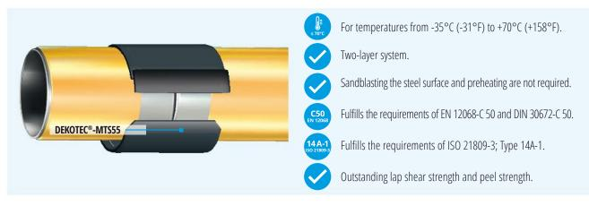
**DEKOTEC®-MTS55** is a heat shrinkable sleeve consisting of an electron beam cross-linked polyethylene backing and a coating on bitumen basis for the corrosion prevention of the field joints at steel pipes.
