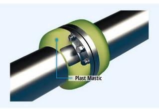
**DENSO®-Plast Mastic** is a hydrophobic mastic filler on petrolatum basis for the **filling of cavities** as well as the **equalization of uneven surfaces** at buried pipeline components (e.g. flanges and armatures). DENSO®-Plast Mastic, due to its reinforcement with filler materials and fibers, permits a **good moldability and stability**.
