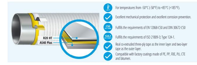
**DENSOLEN®-AS40 Plus/-R20 HT** is a cold applied two-tape system for the corrosion prevention of metal pipes and pipelines in extreme corrosion conditions and mechanical stresses. Compared to the single tape system DENSOLEN®-AS40 Plus, a robust and UV resistant surface of the encasement is achieved with the outside tape **DENSOLEN®-R20 HT**.
