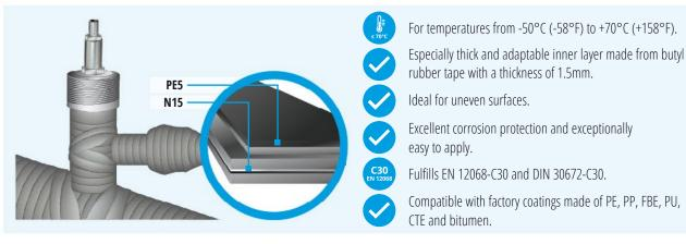
**DENSOLEN®-N15/-PE5** is a cold applied two-tape system for corrosion prevention of metal pipes and moldings with special qualification for the application of uneven substrates and complicated geometries.
