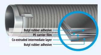
**DENSOLEN®-E** and **DENSOLEN®-N** are plastic tapes that are processed cold. They are butyl rubber based for permanent corrosion prevention encasements and electrical insulations.
