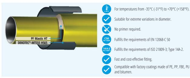
**DEKOTEC®-MTS55 HS65** is a heat shrinkable sleeve with **extreme shrinking capacity**. It is comprised of a robust electron beam cross-linked polyethylene carrier film and a bitumen-based coating.
