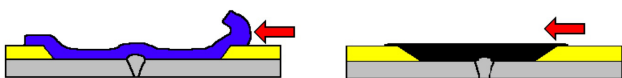
Figure 1. Field joint coating on top of the factory coating (left) and inline with factory coating (right).
