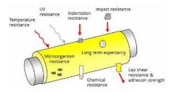
Figure 2. External factors for field joint coating.
