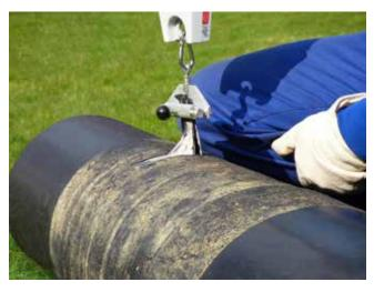
Figure 4. Cohesive separation pattern after 39 years.
